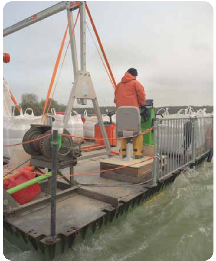
Figure 8. Treatment to a large waterbody using a crane fitted pontoon system. Kralingse Plas, The Netherlands.
