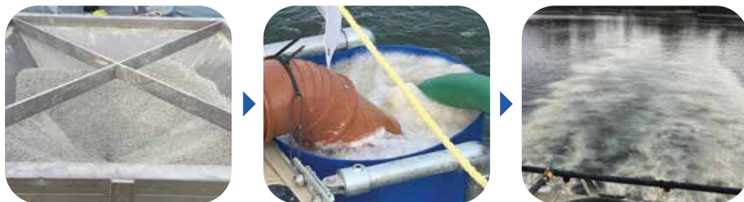
Figure 6. Phoslock® application process, with granules (left) being mixed with lake water (middle) and then applied to the surface of a waterbody (right).
